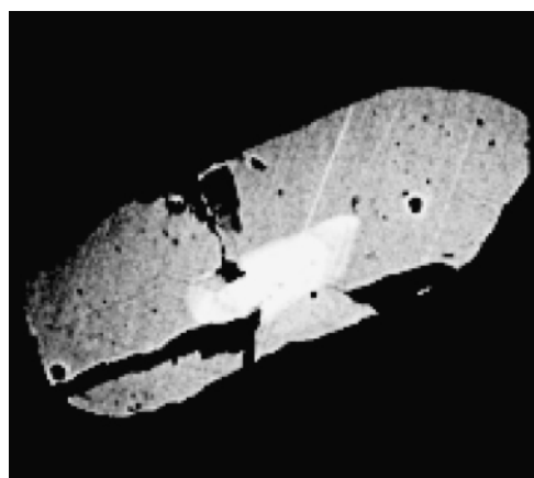
Fig. 4. Back-scattered electron image of zircon separated from the Morven Cabrach gabbro. Field of view 150 \mu\text{m} .
