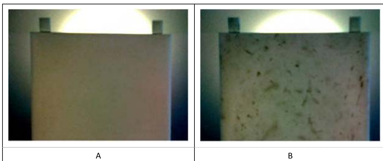
Figure 5.1; Demonstrating a visual test of filler dispersion within concentrates by lowering their concentration to form plaques using an injection moulding process, for two different samples that A) passed and B) failed
