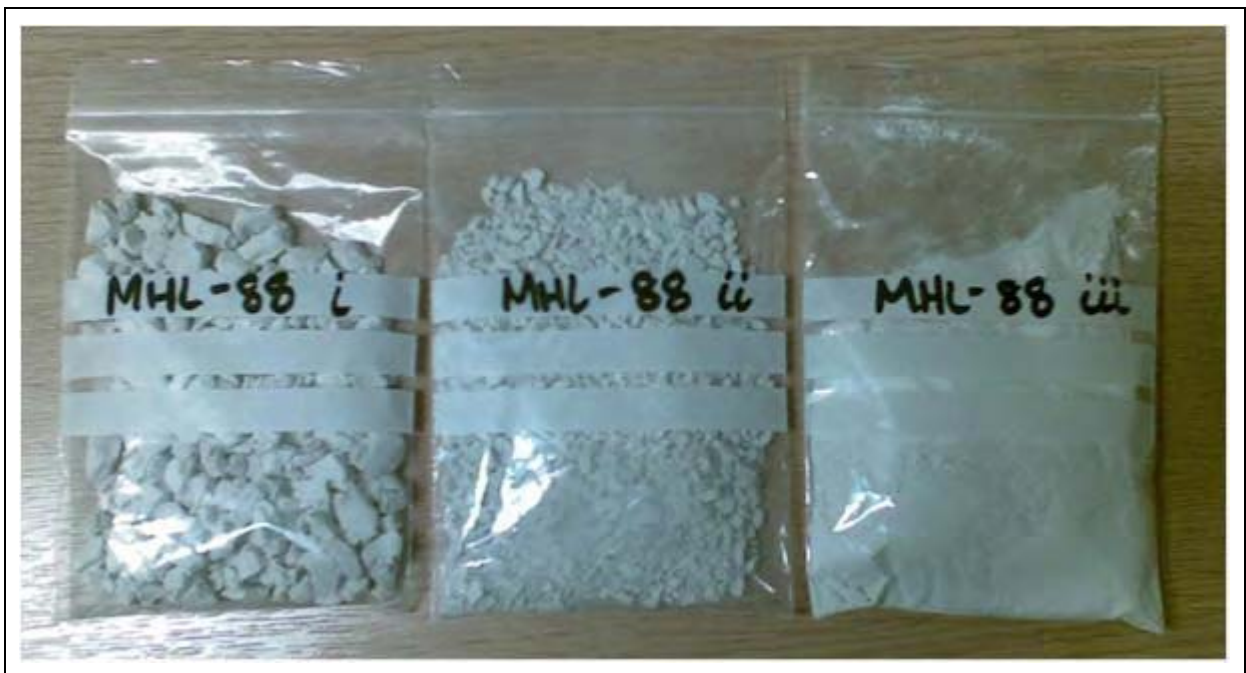
Figure 5.8; Product forms of an 88 % w/w GCC/PE wax concentrate. Diameter (mm) as follows; i) 3.5 \leq d < 9.5 , ii) 2.0 \leq d < 3.5 and iii) 0.0 < d < 2.0
