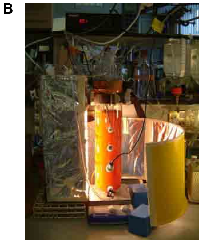
Figure 2.3-a A photobioreactor for the continuous culture of Rhodobacter sphaeroides . Schematic diagram (A) and operational system shown with the reflective tube unfurled (B).
