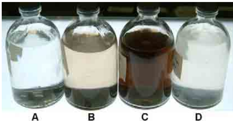
Figure 2.8-c The effect of medium composition on the precipitation of Pd(0).
