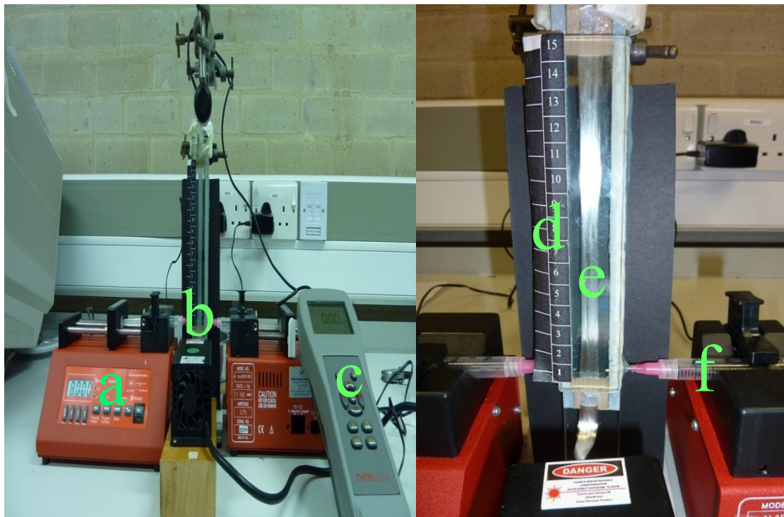
Figure 3.6: Experimental setup – impregnation of E-glass ( a. Automated syringe driver; b. Laser light source; c. Power meter; d. Calibrated unit; e. Assembled composite moulds with fibre bundle ready for impregnation; and f. Injector).
