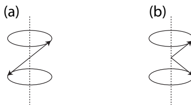
Figure 2.8: (a) Radical electron pairs are initially in a singlet state after the chemical bond is broken. (b) As the two radical electrons precess at different frequencies due to the Zeeman splitting of the attached proton a triplet state can result.
