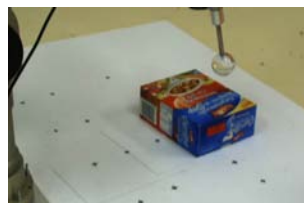
Figure 7.4: Video 3 Tipping : First, the object is pushed so that it is supported by the finger in a partial tipping position (frames 100 and 134, video key frame set 3.1). In the space of a few frames the object becomes unstable and leaves one energy configuration and enters another low energy configuration (frame 141, video key frame set 3.2). If a tracker fails at this point it may yet recover later on so a key frame set is examined about 6 seconds after this initial fall (frame 317, video key frame set 3.3).
