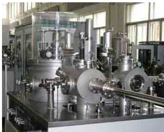
Figure 5.2- UHV multifunction magnetron sputtering system used to deposit the HfO_2 dielectric.
