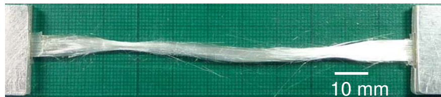
Figure 4.32 A representative image of a fractured silane-treated E-glass fibre bundle specimen.
