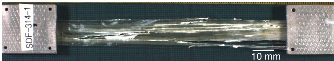
Figure 4.57 Representative image of a fractured as-received SDOF composite.
