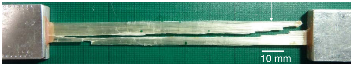
Figure 4.58 Representative image of a fractured heat-treated SDOF composite with an arrow highlighting the region of partial interfacial debonding.
