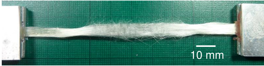
Figure 4.31 A representative photograph of a fractured as-received E-glass fibre bundle specimen.
