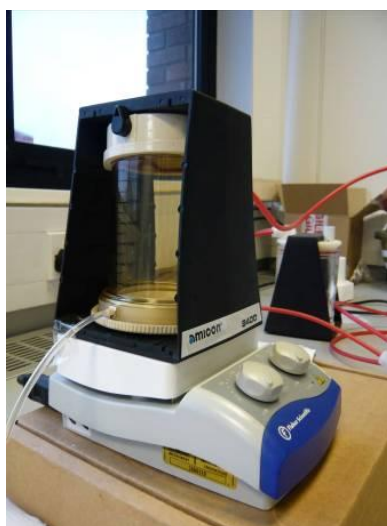
Figure 3.3 Ultrafiltration equipment assembly. Sample is placed in chamber, N 2 gas is passed over the sample from the top with the filtrate collected from the bottom. The sample can be stirred to reduce aggregation as the sample concentrates.
