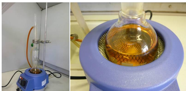
Figure 6. 1 Apparatus used for the refluxing of the reduced silver nanoparticles
