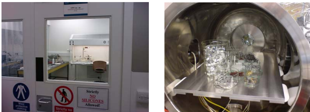
Figure 3.19: Images of Birmingham BOSEM production clean-room facilities. (Left) Dedicated clean-room assembly suite. (Right) Cleaned parts in bake-out oven.
