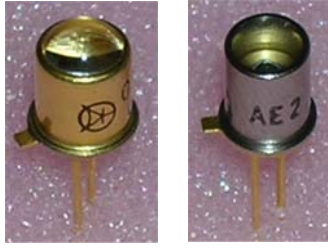
Figure 3.10: Images of leaded sensor components.
