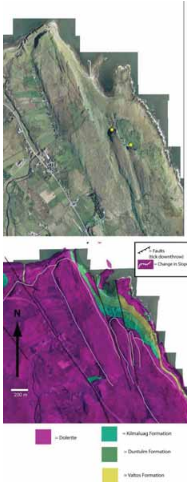
Fig. 4.9 – Aerial photograph and aerial photograph draped with BGS 1:50000 solid rock geology map. The BGS interpretation places faults coinciding with the troughs between the finger structures at Staffin. No evidence of faulting can be seen within the fore-shore area of the harbour and no apparent offset occurs in the top surface of the dolerite forming the fingers.
