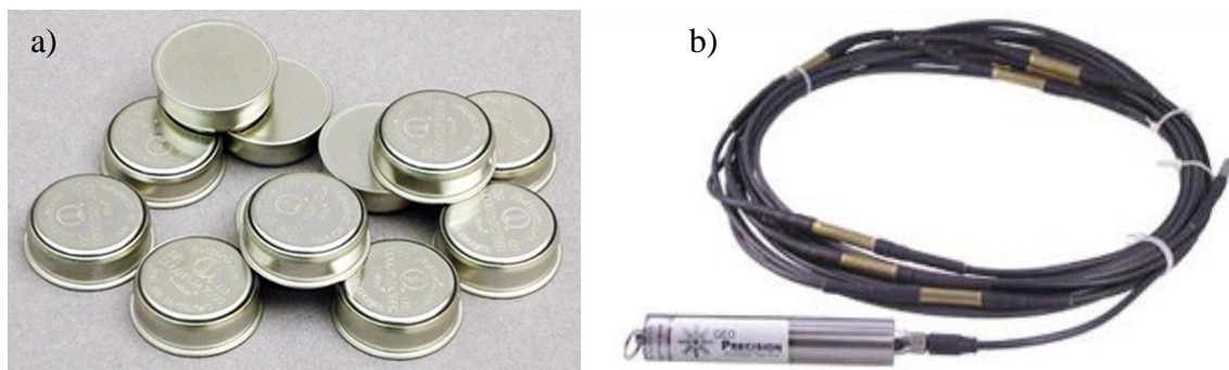
Figure 18. a) iButton ground/air thermistors. b) Ground temperature GeoPrecision thermistor strings.
