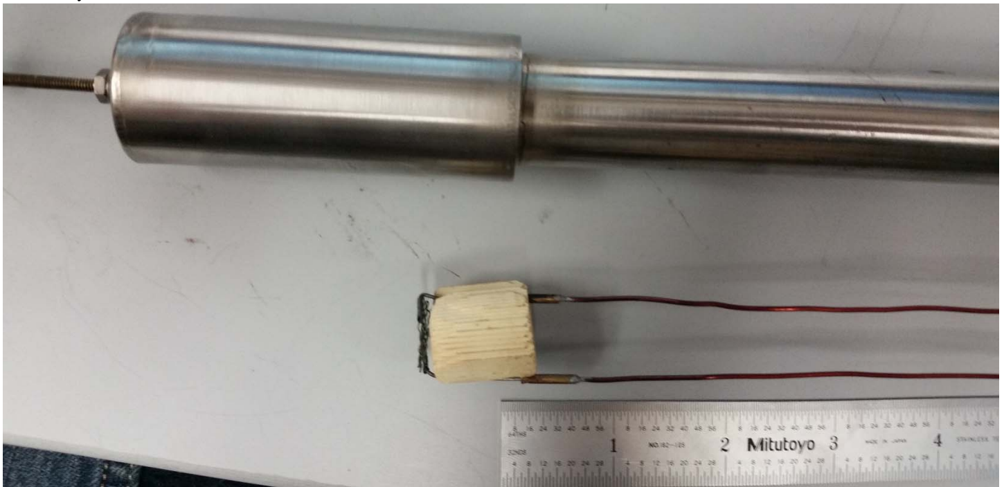
FIGURE 4: TAPS BODY WITH ELECTRICAL HEATER WIRE AND STACK, NEXT TO SCALE.
