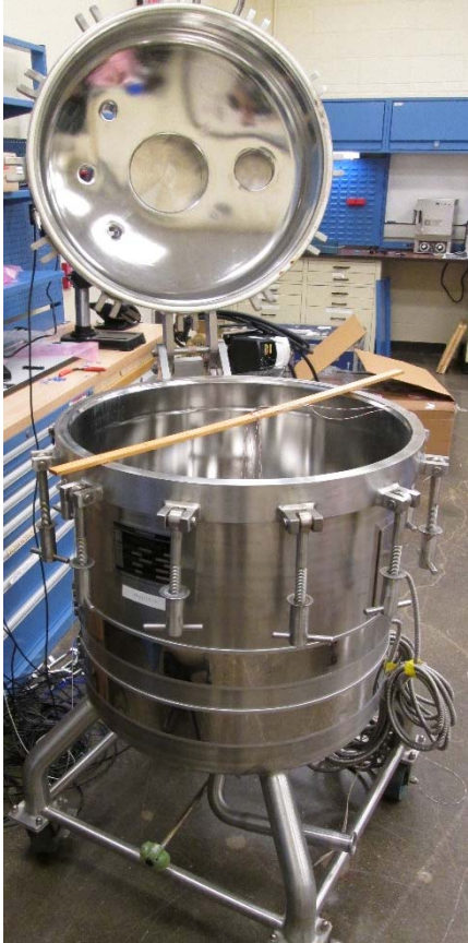
FIGURE 7: TEST VESSEL WITH OPEN LID. METER STICK IS USED TO SUSPEND TAPS INSIDE VESSEL.
