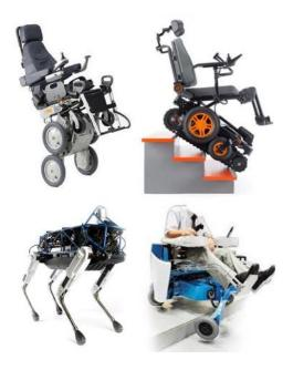
Figure 1: Mobility-Robotic designs, wheeled (top-left), tracked (top-right), legged (bottom-left), and hybrid legged-wheel (bottom-right) robots
