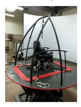
Figure 7: Experiment Setup: MEBot on the CAREN system
