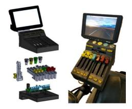
Figure 25: 3d model exploded view of the ACG Interface (Left), ACGI mounted in the MEBot wheelchair (right)
