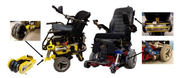
Figure 15: Mechanical improvements of MEBot2.0 (right), and MEBot2.5 (left)
