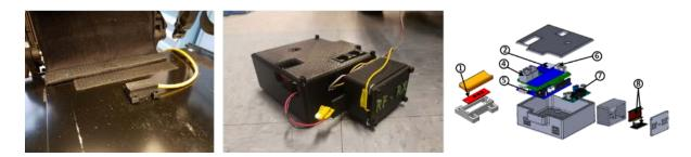
Figure 17: IMU sensor located under the seat of the wheelchair (Left), DAQ board assembly (Center), Exploded view of the Data acquisition board (Right)
