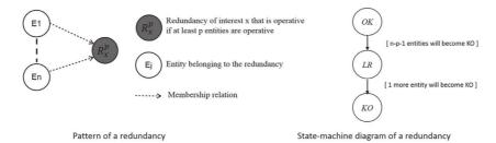
Fig. 5. Pattern and state-machine diagram of a redundancy.
