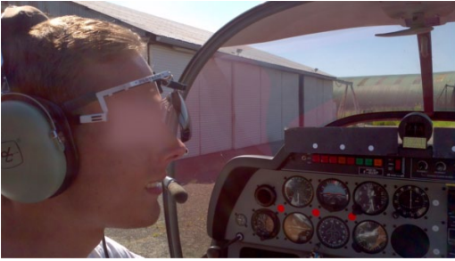
Figure 3. Pilot with eye-tracking setup on board of a DR400 light aircraft.
