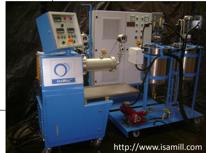
Attrition reactor ~4 L operating under T (max 200°C) & P (max 30 bar)
