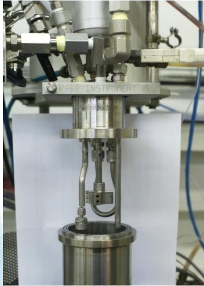
Stirred mill (self-built): 300 mL, batch, 120-180°C, 20bar CO 2
