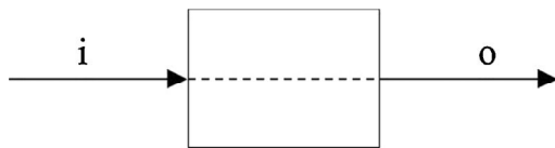
Fig. 5. Simple unit operation (1 input–1 output) (‘SISO’ system).
