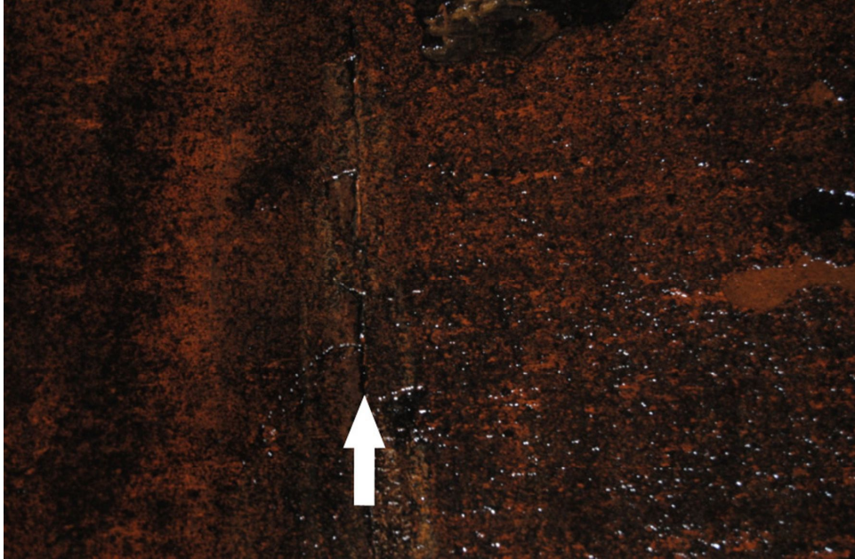
Fig. 3. Biofilm on the galvanized steel (left) and the concrete part (right) of the HP site. The white arrow shows the separation between both zones.
