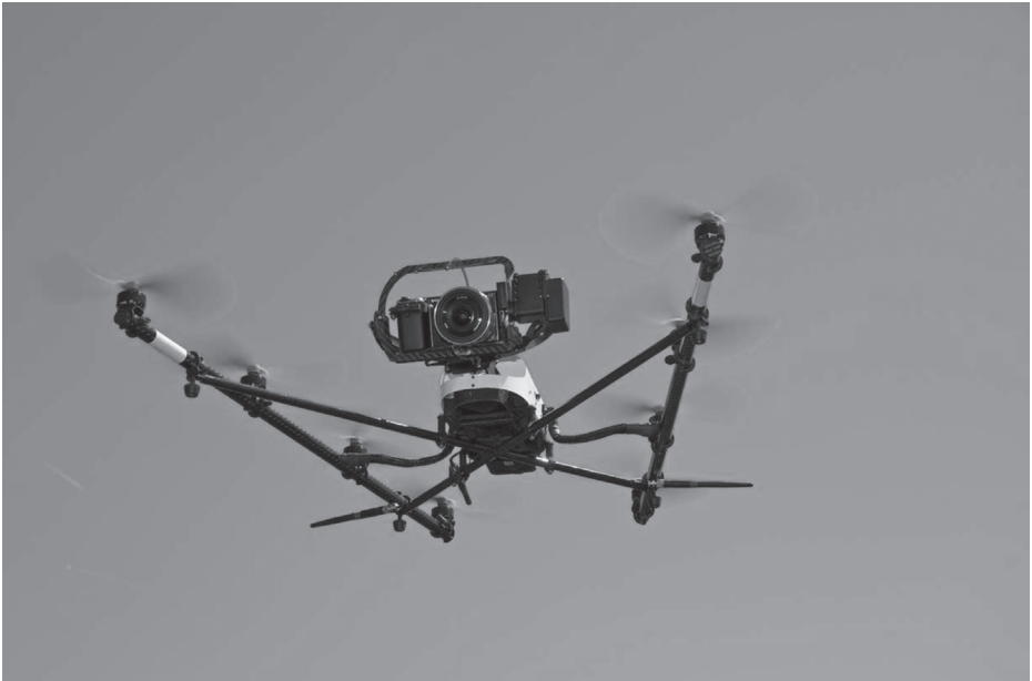
Figure 1.7 An eight-rotor mini-UAV developed by Ascending Technologies (photo credit: Lakeside Labs GmbH)
