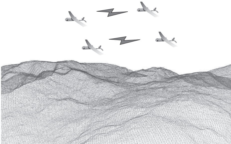
Figure 1.18 Multiple UAVs forming an aerial mobile ad hoc network
