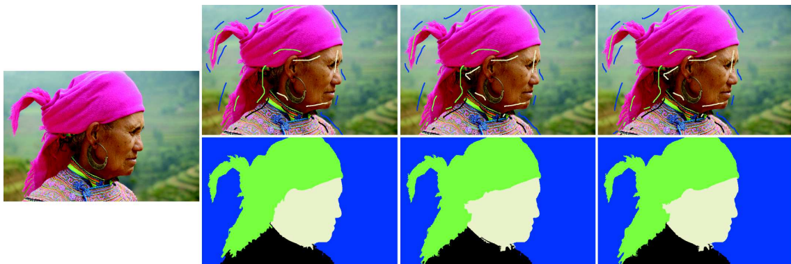
Fig. 14 SaF seed evolution example for a problem with four classes. Only two updates of seeds are required to achieve an accurate result.
