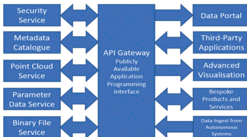
Fig. 1 - An overview of the iMarDIS architecture showing the 'back end' microservices to the left of the Application Programming Interface and the applications domain on the right handside. The applications domain is where advanced service capability can be implemented either by iMarDIS or third party developers.
