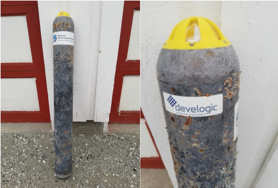
Fig. 4: Original DW.SRB before improvement (plastic cover possibly degraded antenna performance)
