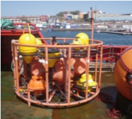
Fig. 8: The MYRTLE-X lander following recovery from trials in early 2018. The orange painted aluminium frame provides the structure with orange, hard-hat covered glass spheres in the middle of the frame providing buoyancy. The MYRTLE electronics are housed in smaller glass spheres spread around the bottom
