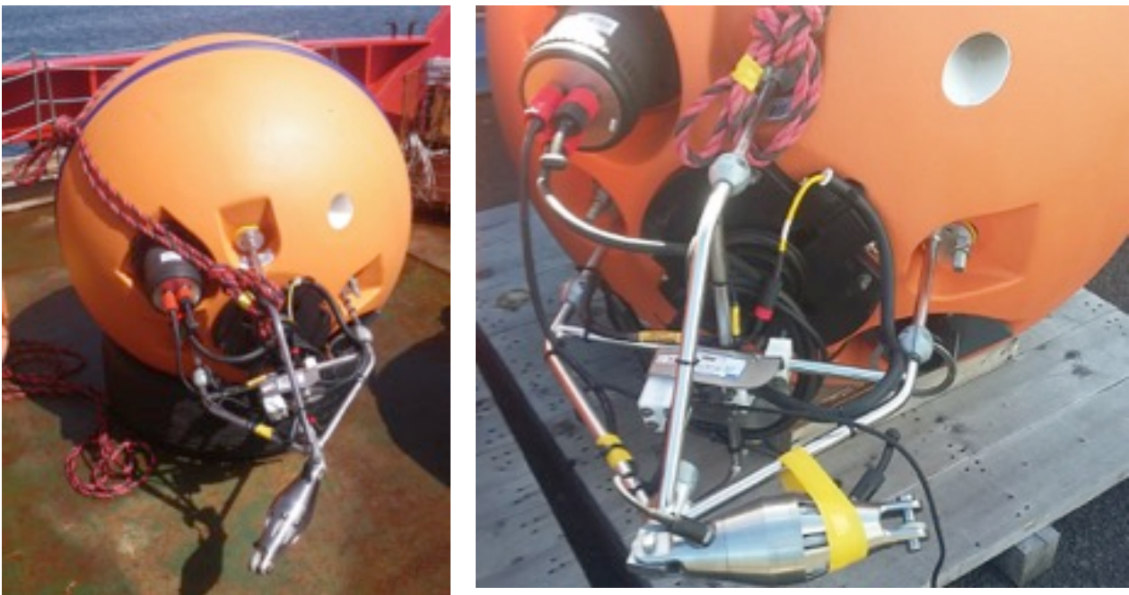
Fig. 7: (Left) - The syntactic float telemetry buoy following recovery from trials in early 2018 (left). Right – a close up showing the components. The dark grey pressure case on the left houses the mooring controller electronics; in the black central clamps is the Benthos moored acoustic modem and batteries; in this float the acoustic modem transducer is mounted opposite the mooring controller (just visible behind the float metalwork) and is therefore pointing down for use with the MYRTLE-X lander; mounted to the cross bars of the float metal work is the Sea-Bird inductive coupler through which an electrical cable passes – this cable is connected to the inductive swivel mounted to the framework at the bottom of the picture with the other end of the swivel connecting to the mooring wire.
