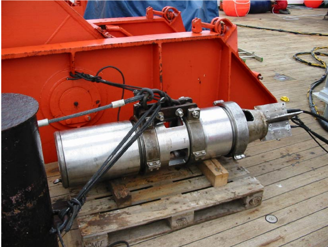
Fig. 2.10: One of the 32 litre guns on deck
