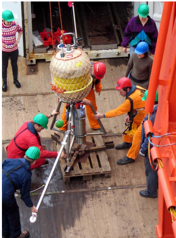
Fig. 2.7: Tripod OBS after recovery being readied for next deployment
