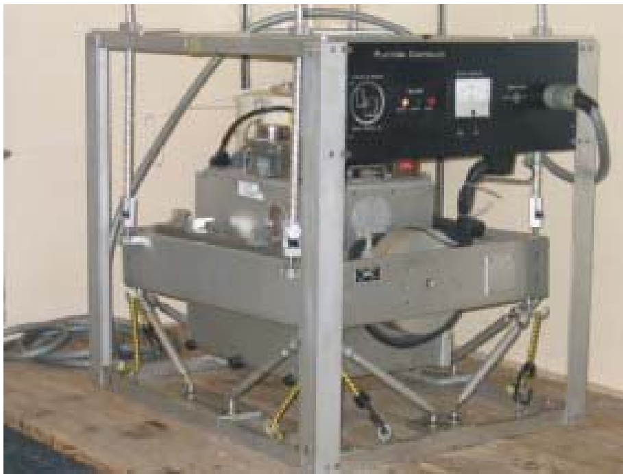
Fig. 2.12: Photograph of the Gravimeter installed in Cork.
