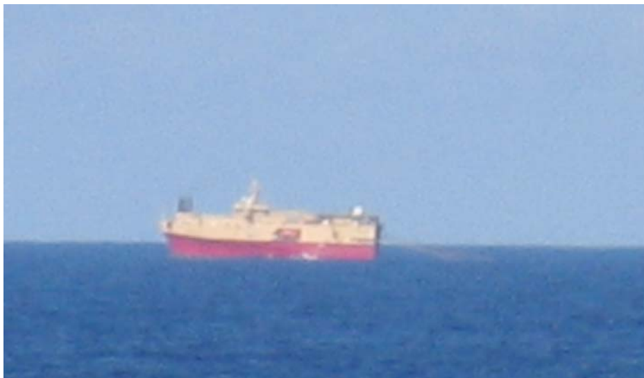
Fig. 2.4: Photograph of the RAMFORM VALIANT, about 3 miles away. The 12 streamers (each 6 km long) can be seen at the stern – the tailbuoys were also clearly visible from Meteor
