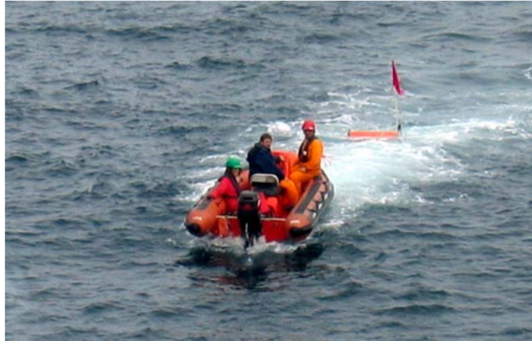
Fig. 2.3: Recovery of the “Walze” OBS. The instrument was successfully dredged with a cable and recovered by boat
