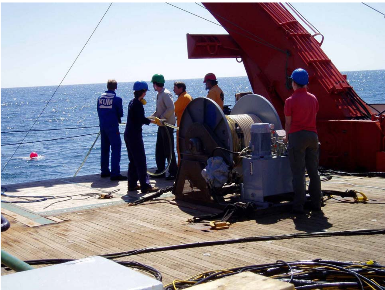
Fig. 2.9: Deployment of the mini-streamer
