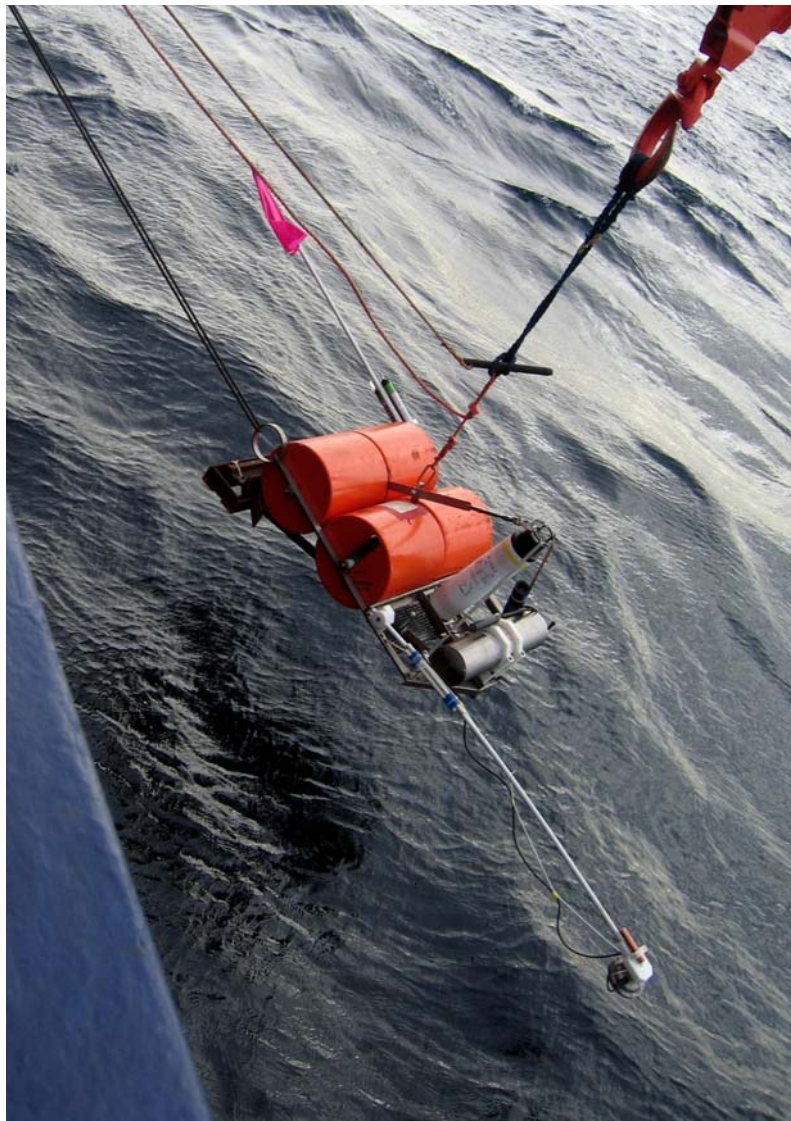
Fig. 2.8: Deployment of “Walze” (“Roller”) ocean bottom seismometer. These instruments are designed to lie flat on the seafloor (reducing noise from currents), but to rotate to vertical when released. The geophone arm can be seen to the bottom right.
