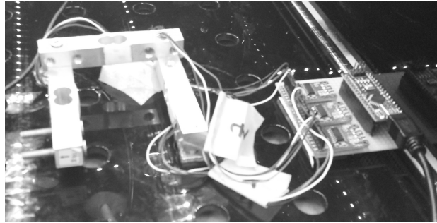
Fig. 7 The force measurement system under the phantom
