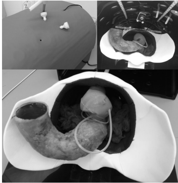
Fig. 3 The first prototype of the laparoscopic trainer box with the pelvic phantom
