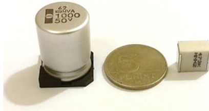
Fig.5. LN0 (left) and 4036 (right) sized SMD capacitors.
