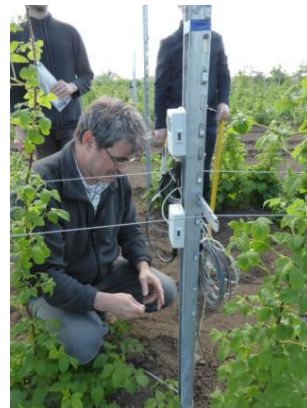
Figure 3: Temperature sensors at: - 0,15 [m], 0 [m], 1,0 [m], 1,8 [m].
