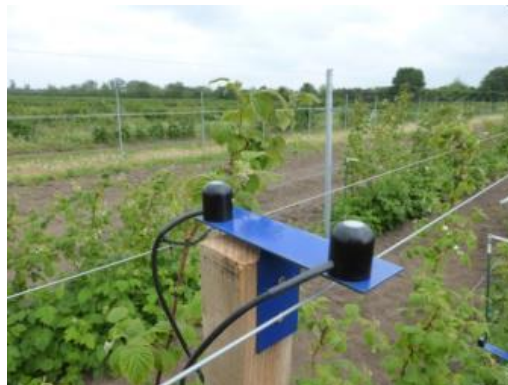
Figure 2: PYR Apogee SP-110 360-1120 [nm] and PAR Apogee SQ-100 380-720 [nm]
