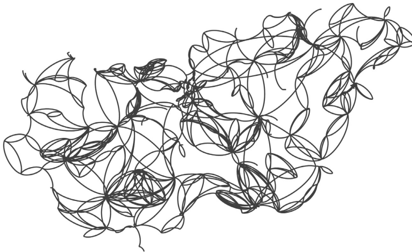
Fig. 4. Hungarian power grid topology (where the load of electric wires is greater than 10 kV; average path length = 3.74).
