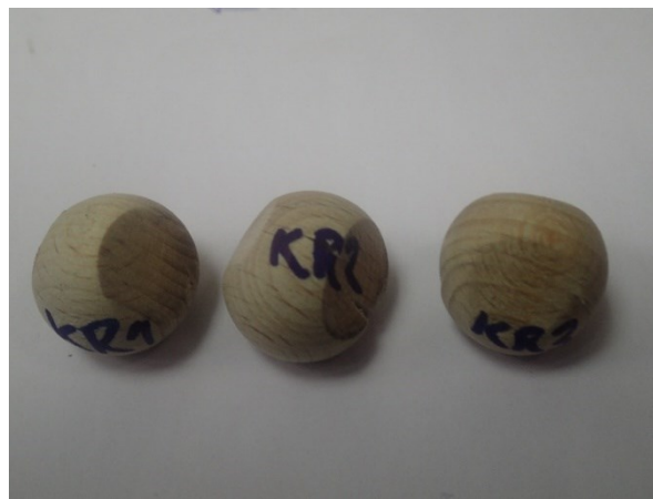
Figure 6. The set of beech balls (KR 1 – 3) after pressing in direction parallel to growth rings.
