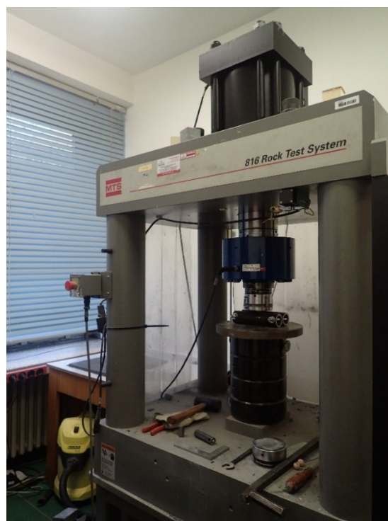
Figure 4. View of used press (type MTS 816 Rock Test System)
