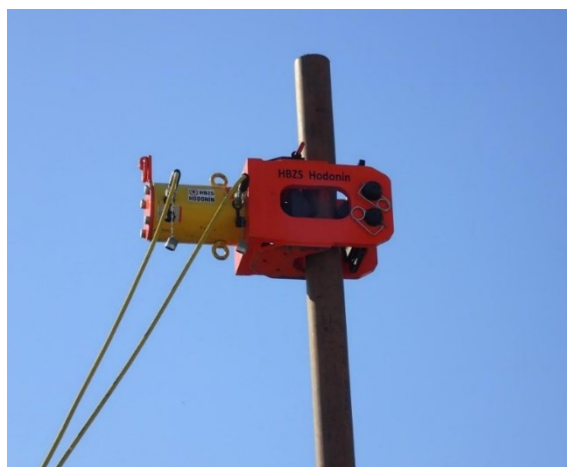
Figure 2. The view of special elimination apparatus FIB-1, fitted on drill pipe. The test in pilot work conditions, area of HBZS Hodonin.
