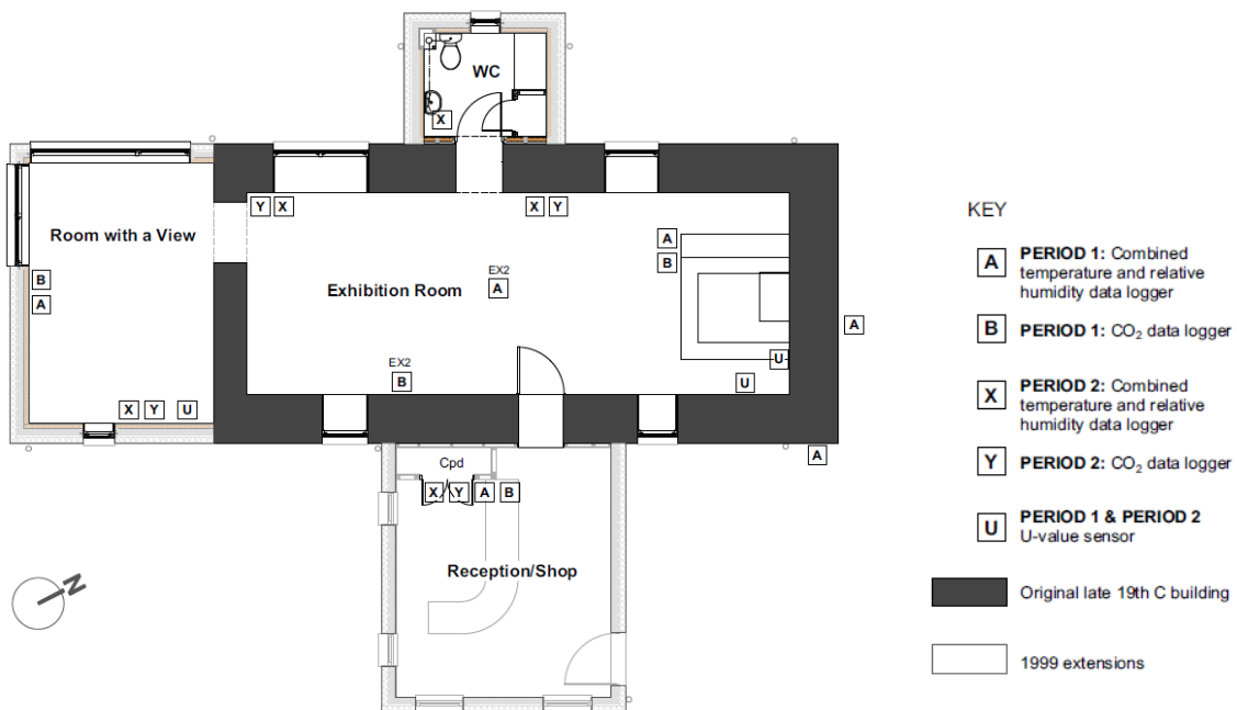
Figure 3. Plan view of LSIC building, indicating the historic core, 1999 extensions and location of monitoring apparatus for PERIOD 1 and PERIOD 2 BPE.
