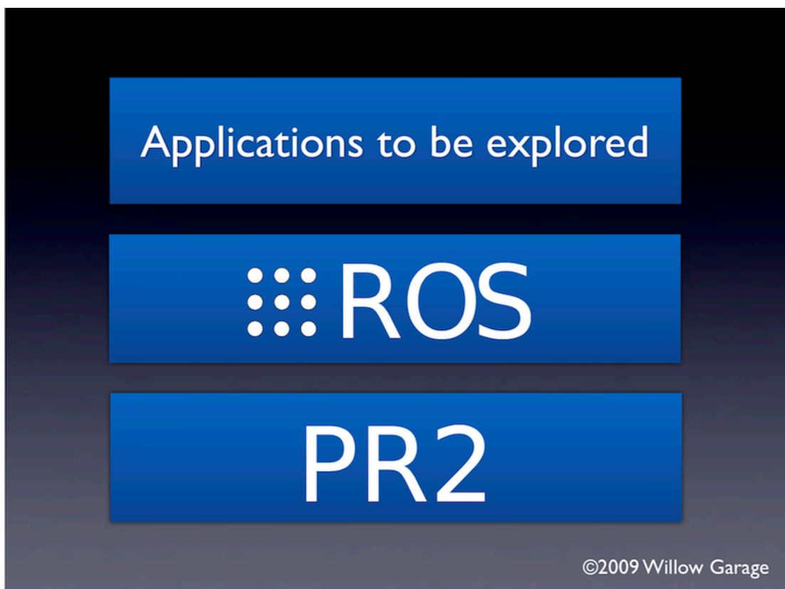
Figure 11: PR2, ROS and applications as a layered stack 11
