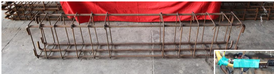
Reinforcement Cage Longitudinal bars all 20 mm diameter (Inset: Packaged FBG tied to bar)
