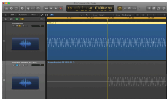
Figure 6. Observing delay between the source and returned audio streams to determine round-trip network latency, using Logic Pro X software.
