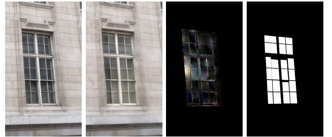
Figure 14: From left to right: input cropped image, extracted diffuse layer, extracted variation layer (intensity), reprojected reflection mask.
