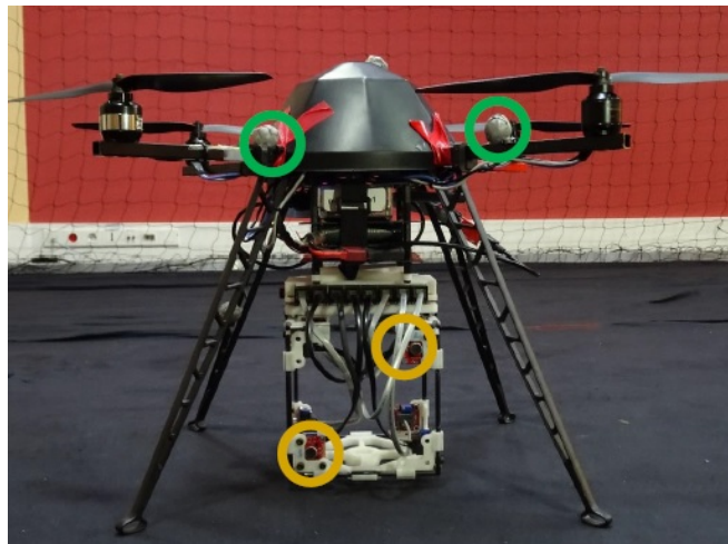
Fig. 1: The MikroKopter quadrotor UAV used for the DREGON dataset, with our 3-D printed 8-channel microphone array mounted on the bottom. Green circles highlight two of the passive markers used for motion capture and yellow circles highlight two of the microphones (best seen in colors).
