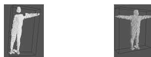
Figure 3: A depth first (left) and width first (right) octree carving with the same elapsed time. The former leads to an unbalanced space carving, the latter to a balanced one.
