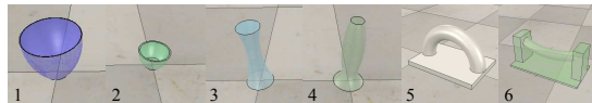
Figure 3. Objects used to learn multiple grasp types: objects 1 and 2 were used for precision grasps, objects 3 and 4 were used for power grasps, and objects 5 and 6 were used for medium-wrap grasps.
