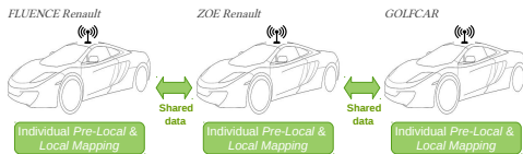
Fig. 1. Scheme of our CoMapping System considering a decentralized case
