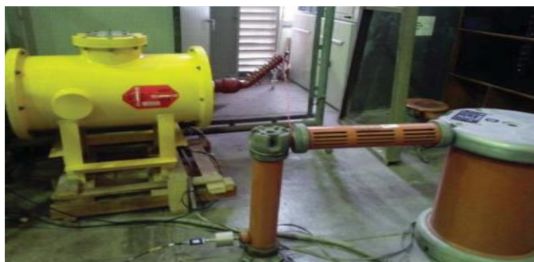
Figure 31 Partial Discharge measurement circuit (Khayam & Vauzia, 2014).
