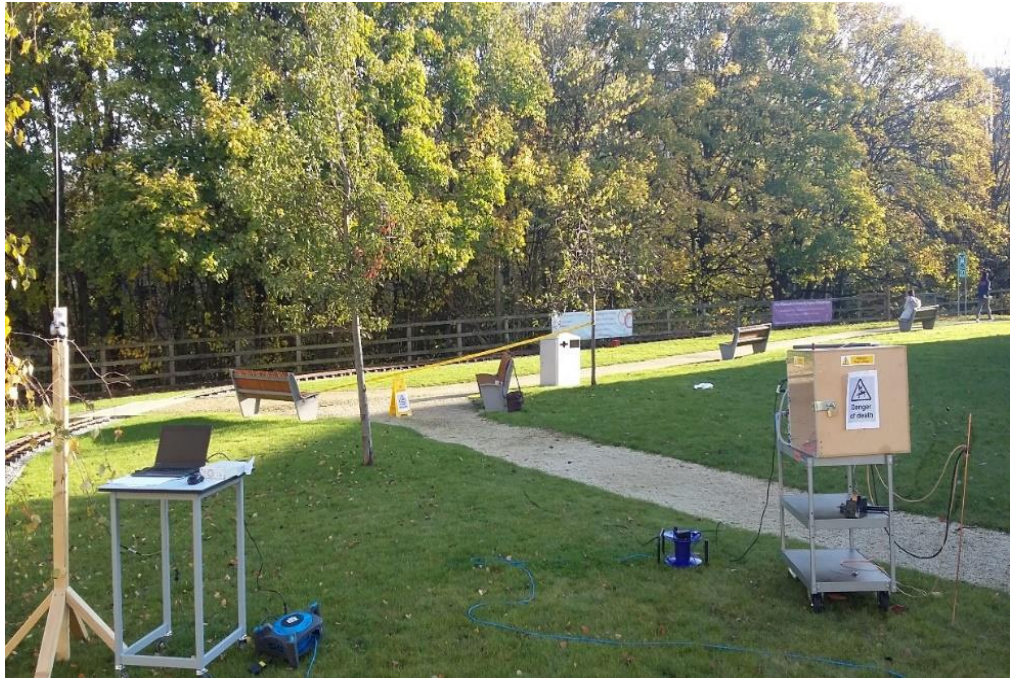
Figure 76. PD measurements using two systems. (SDR and radiometric).
