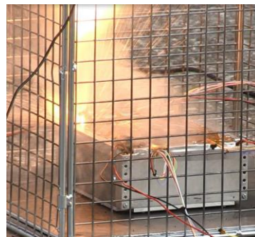
Figure 13. Test Battery induced into thermal runaway
