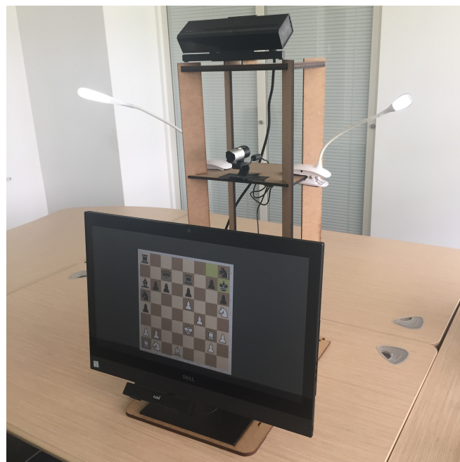
Figure 2. The experimentation equipment used for data collection. On top, a Kinect2 device looking down at the player. In the middle, a webcam to capture the face. At bottom, the touch screen equipped with an eye-tracker presenting the chess game. These views are respectively at left, right and center of Figure 1. The wooden structure is rigid to fix position and orientation of all sensors. The lighting conditions are controlled by 2 USB LED lamps on the sides.
