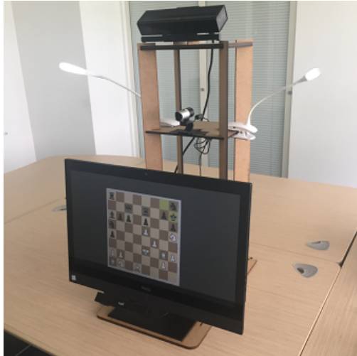
Figure 1: Instrument for recording gaze and emotions of experts engaged in solving problems. On top, a Kinect2 oriented at the player. In the middle, a USB camera to capture the face. Illumination is provided by two LED lamps on the sides. A wooden structure is used to provide a fixed position and orientation for all sensors.
