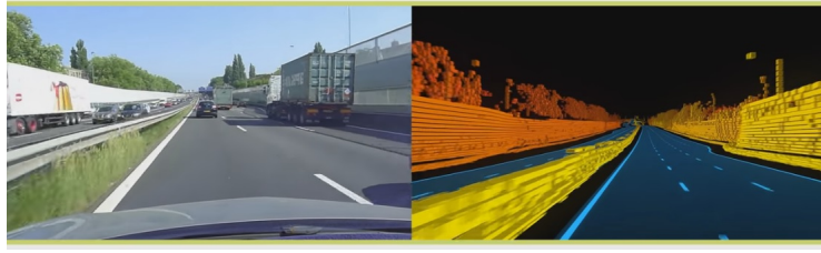
Fig. 1. Example of High Definition (HD) map from TomTom RoadDNA (Reproduced with permission of the copyright owner)
