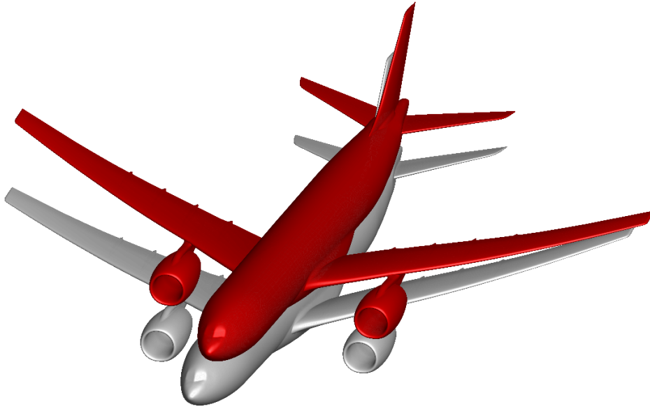
Figure 2.2: Mode shape resulting from eigenvalue analysis. It is a linear combination of both translation and rotation.
