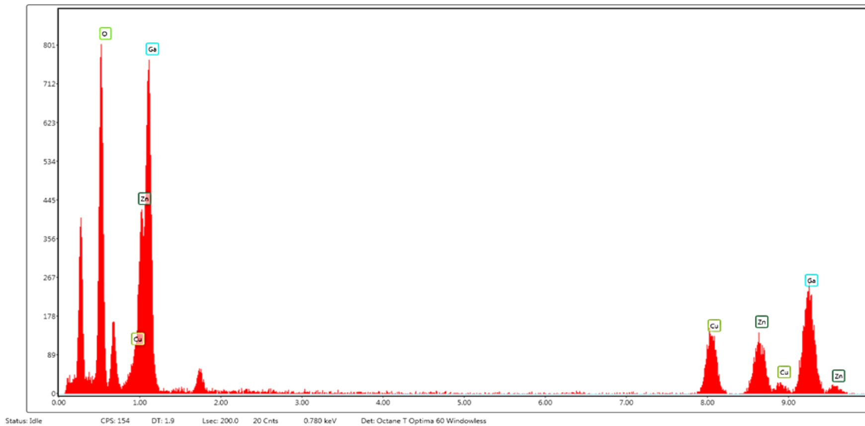
Figure 3.4: Energy-dispersive X-Ray spectroscopy (EDX) of ZGO:Cr crystals.
