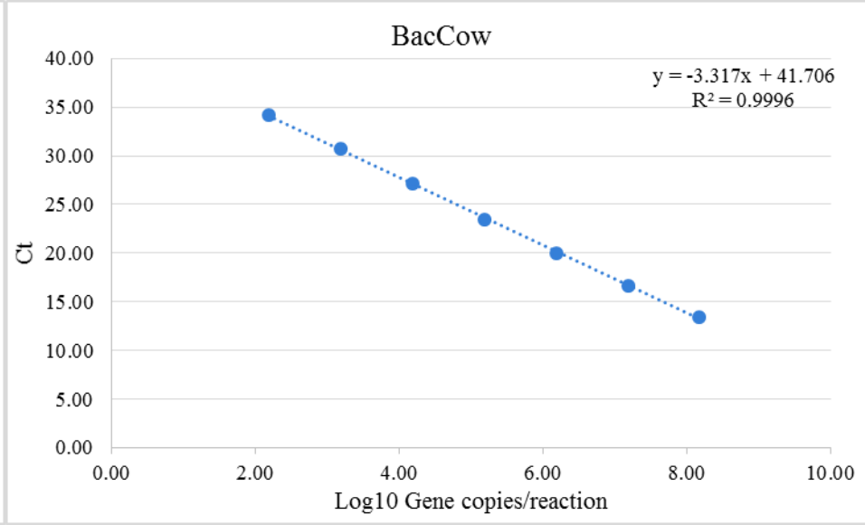
Fig.S4.1B Standardized master standard curve for MST assays: Human (HF183 SYBR, Hum2), swine (Pig-2-Bac) and livestock associated (BacCow) assays
