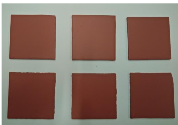
Figure 5.2. 5cm x 5cm PVC plates coated with the pristine paint and the nanocontainer-doped paints, used for the antibacterial tests.
