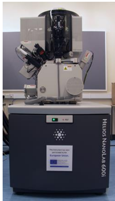
Figure 2.7. FEI Helios Nanolab 600i dual-beam FIB-SEM used for the cross-sectional images of pristine and nanocontainer-doped paints.
