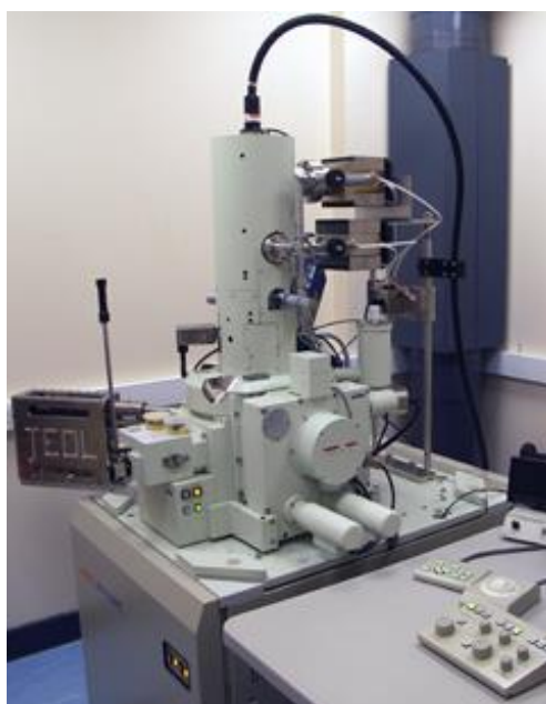
Figure 2.1. Photograph of the JEOL JSM-7001F scanning electron microscope used for the SEM measurements.
