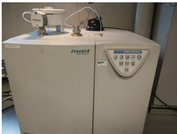
Figure 2.5. FlashEA 1112 Analyzer by Thermo Fisher Scientific used for the elemental analysis of pristine and modified MCM-48.
