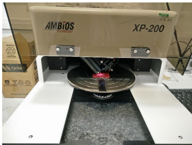
Figure 2.9. Ambios XP200 contact stylus profiler used for the surface roughness measurements of coated PVC plates.
