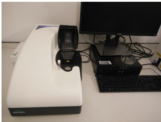
Figure 2.4. Malvern Zetasizer Nano ZS used for the \zeta -potential measurements of colloidal nanoparticles.
