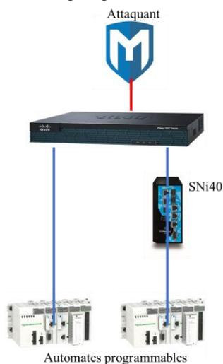
Fig 3. Architecture incluant un IPS SNi40
