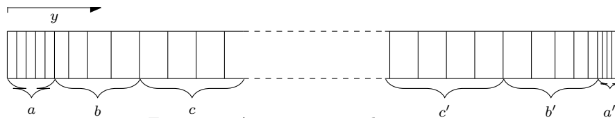
Figure 2 – Asymmetric mesh construction
